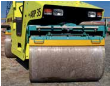
Flexible working width 1100 – 1924 mm
